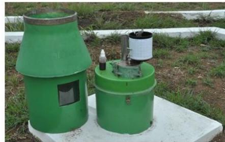
**FLOAT TYPE SELF RECORDING RAIN GAUGE**
