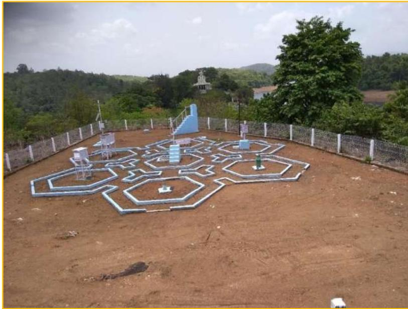
The station is equipped with the instruments for measuring manually the weather parameters namely Atmospheric Pressure, Temperature, Humidity, Rainfall, Evaporation, Wind speed, Wind direction and Bright Sunshine. As part of modernization, an automatic weather station was installed in June, 2014.
