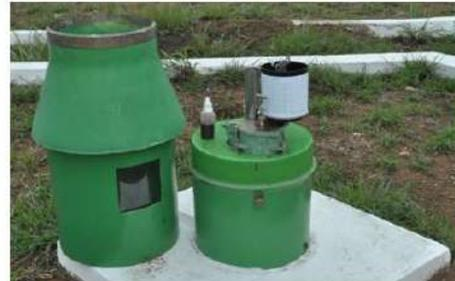
**FLOAT TYPE SELF RECORDING RAIN GAUGE**
