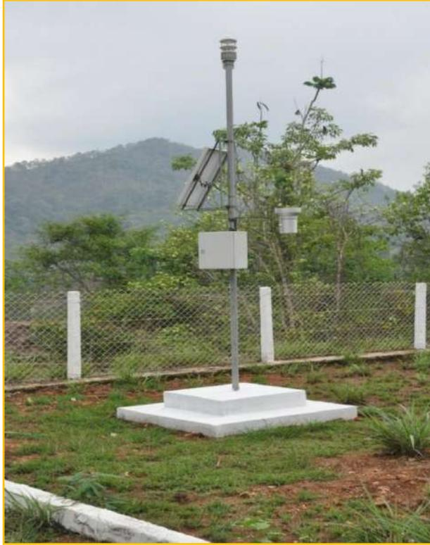
The Automatic Weather station collects data related to Air Temperature, Air Humidity, Barometric pressure, Ultrasonic Wind speed, Ultrasonic Wind Direction, Global radiation and Precipitation using different sensors. These data can be accessed via internet using a software HYDRAS. The data collected can be used to gauge current weather conditions and to make weather forecasts like temperature high/low, cloud cover and the probability of precipitation.
