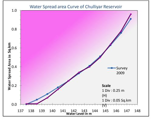
Fig.42 Water level v/s water spread area curve
