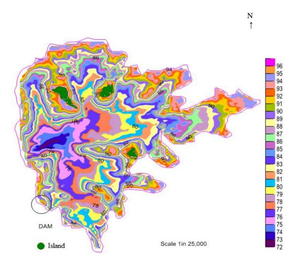
The contour map of water spread area is shown in Fig 17 at an interval of 1m
