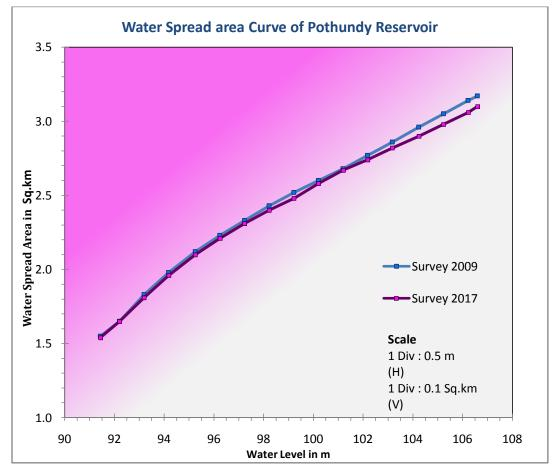
Fig.31 Water level v/s water spread area curve
