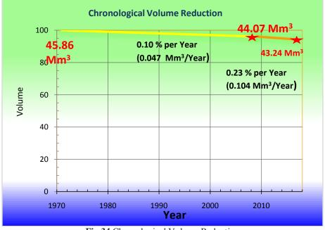
The graphical representation of reduction and rate is shown in Fig.34
