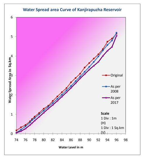
Fig.19 Water level v/s water spread area curve
