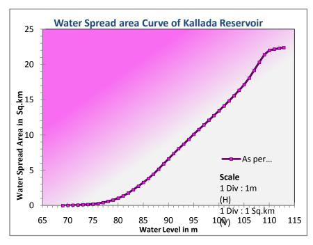
Fig.51 Water level v/s water spread area curve
