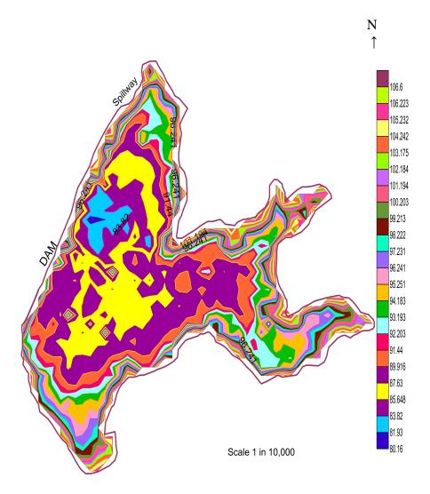
Fig.29 Contour Map based on IBS Survey
