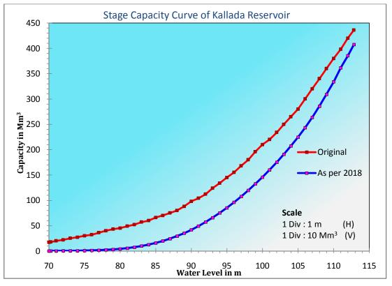
Fig.50 Water level v/s water holding capacity curve
