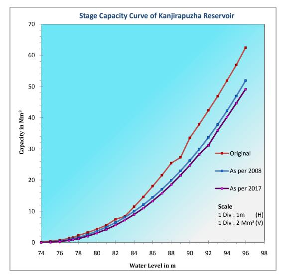
Fig.18 Water level v/s water holding capacity curve
