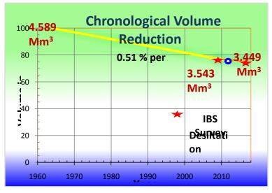
The graphical representation of reduction and rate is shown in Fig.43
