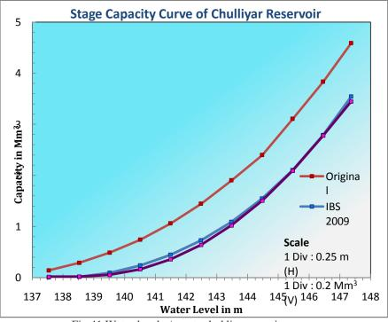
Fig.41 Water level v/s water holding capacity curve
