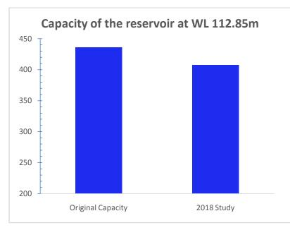
Fig.48 Comparison of Reservoir Capacity at Water Level 112.85m
