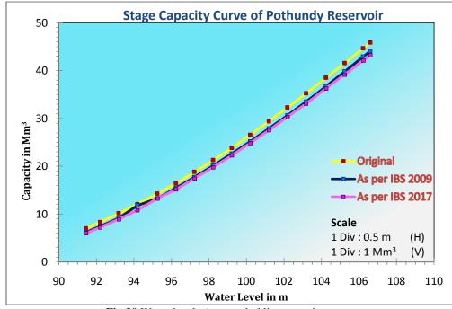
**Fig.30** Water level v/s water holding capacity curve
