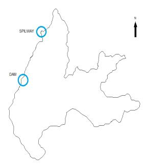
Fig.27 Water Spread Area Map of Pothundy Reservoir at WL 106.6m(surveyed portion)
