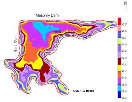
Fig.40 Contour Map based on IBS Survey
