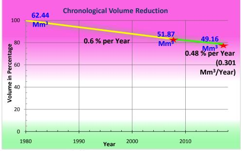
The graphical representation of reduction and rate is shown in Fig.23
