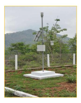
The Automatic Weather station collects data related to Air Temperature, Air Humidity, Barometric pressure, Ultrasonic Wind speed, Ultrasonic Wind Direction, Global radiation and Precipitation using different sensors. These data can be accessed via internet using a software HYDRAS. The data collected can be used to gauge current weather conditions and to make weather forecasts like temperature high/lows, cloud cover and the probability of precipitation.
