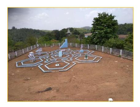
The station is equipped with the instruments for measuring manually the weather parameters namely Atmospheric Pressure, Temperature, Humidity, Rainfall, Evaporation, Wind speed, Wind direction and Bright Sunshine. As part of modernization, an automatic weather station was installed in June, 2014.
