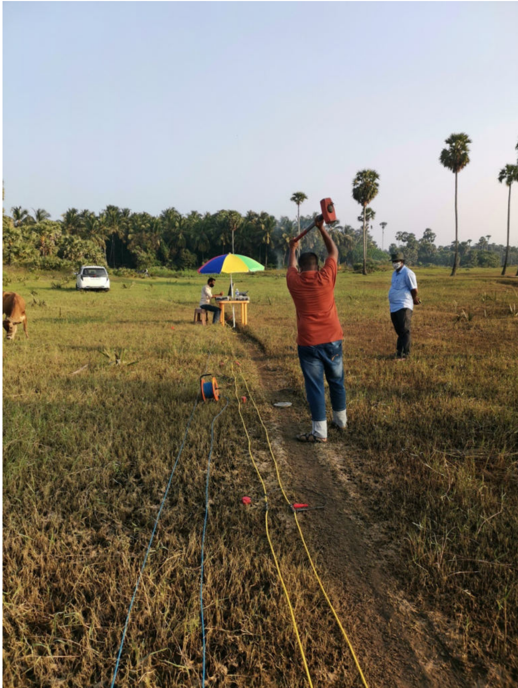
Fig 13. Seismic refraction survey at VenkalakayamEri
