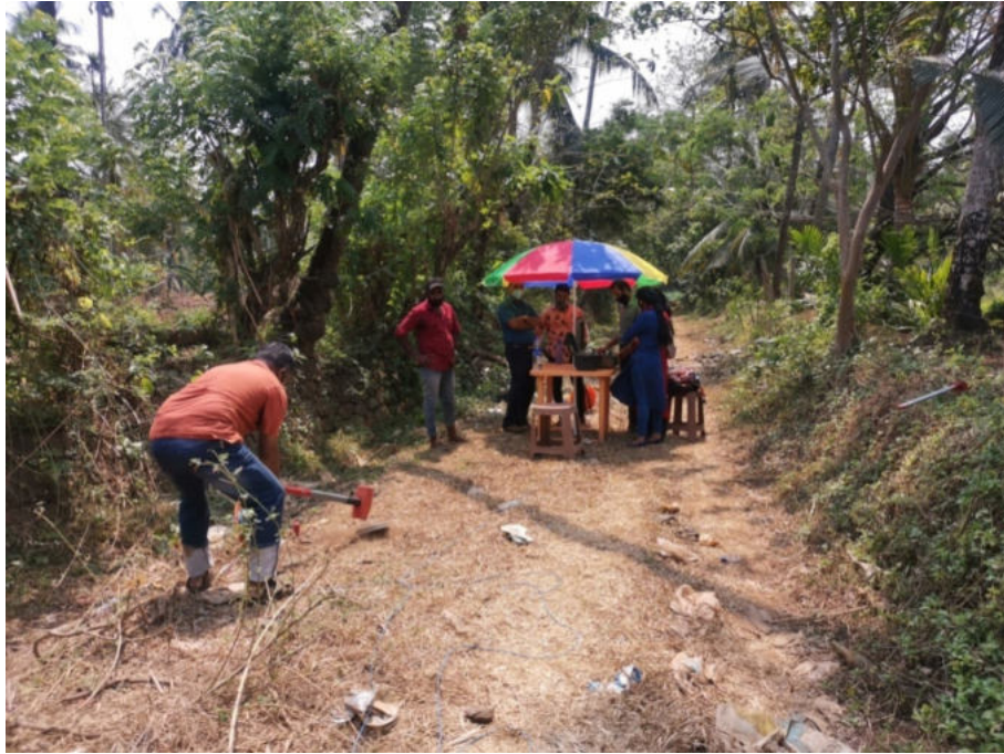
Fig 9. Seismic refraction survey at Alppara
