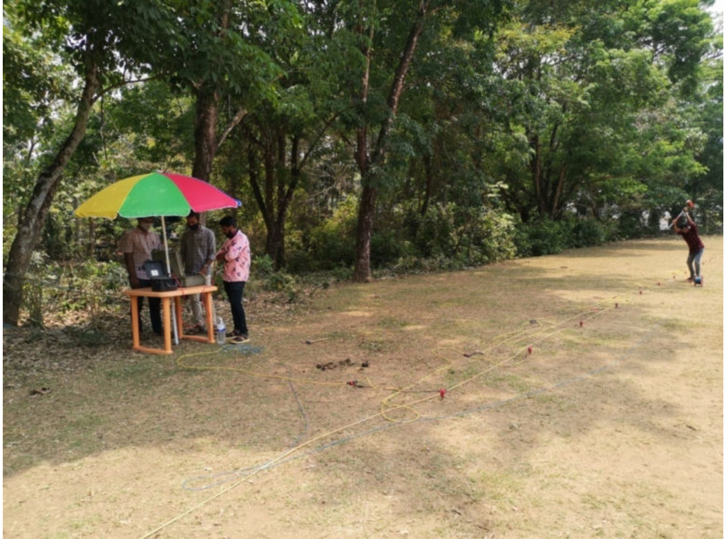
Fig 11. Seismic refraction survey at Echippara Ground
