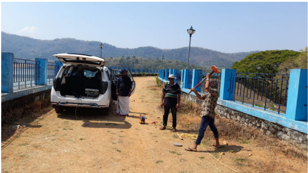
Fig 12. Seismic refraction survey at Chimoni Earthen Dam
