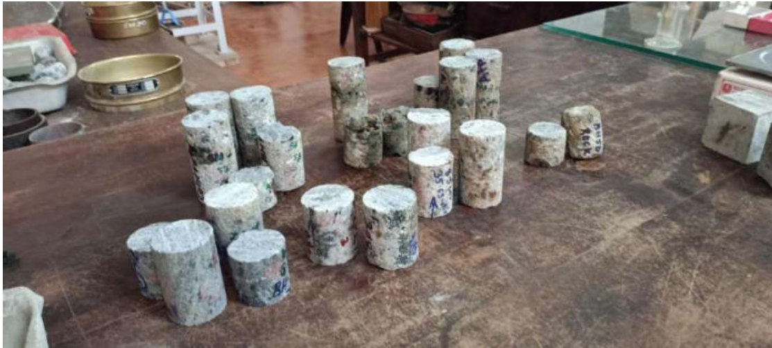
Concrete core samples collected from Attappilly RCB and preparing for testing
