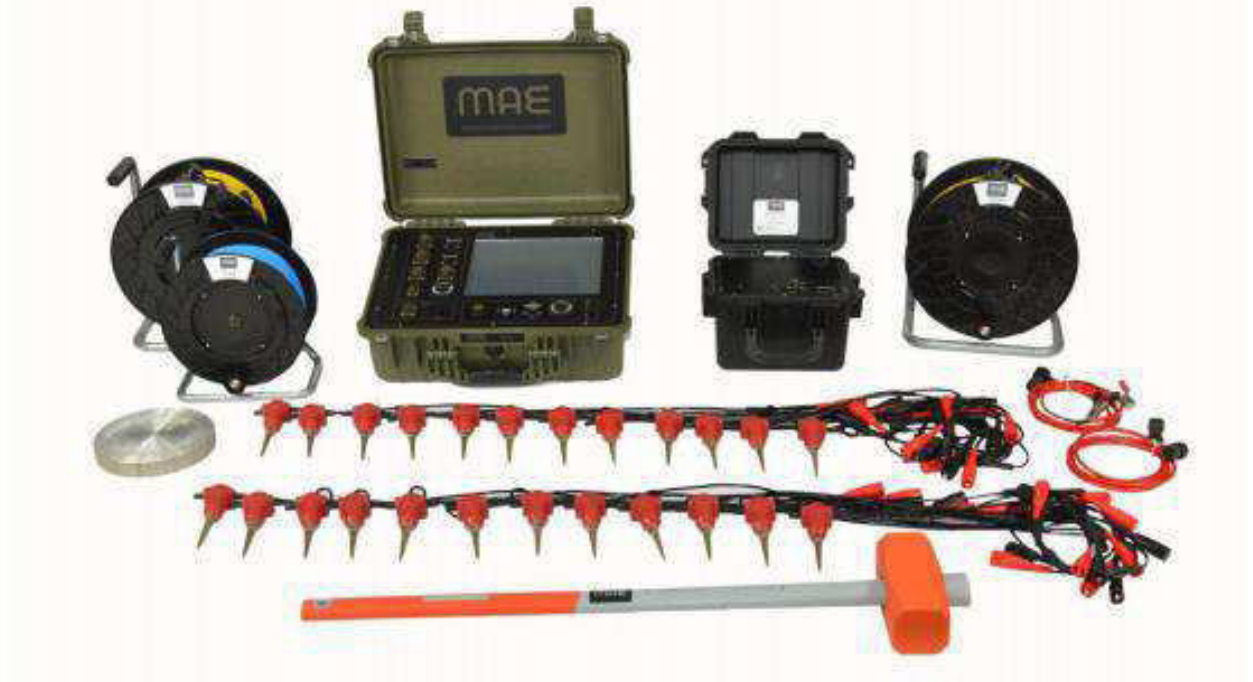
Fig 8. Apparatus used for Seismic Refraction Survey
