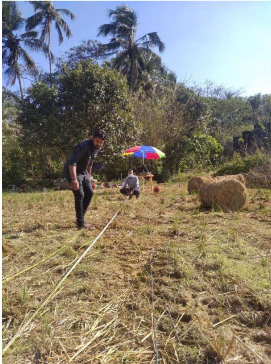
Fig. Seismic refraction survey at Thathanampully
