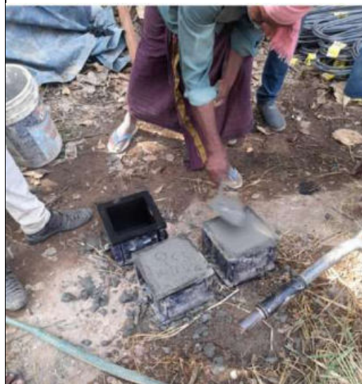
Cube samples From side protection wall of Killiyar Irrigation Section, Thiruvananthapuram
